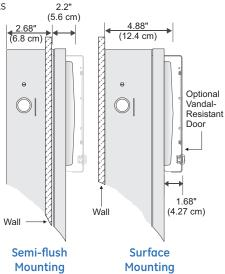
Semi-flush mounting requires an optional trim ring, which adds ¾" to all sides of the panel.
